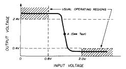
fig. 2. Transfer characteristics of the TTL NAND gate.
